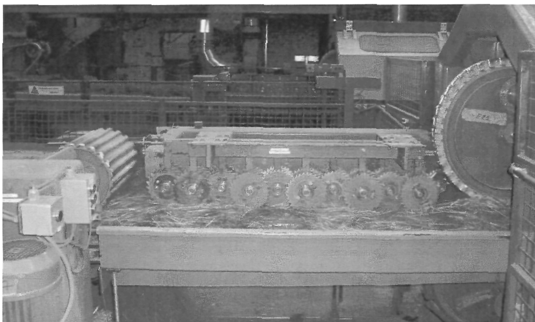
Modern flax-braking by machine, Albert Brille, N.V., Wewelgem, Belgium.
