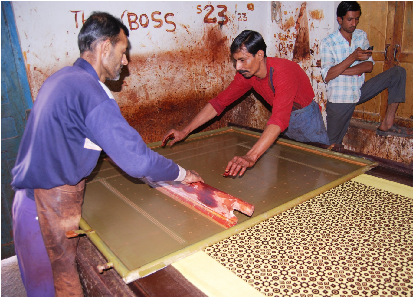
Figure 4 Screen printing ajrakh at Khavda.
