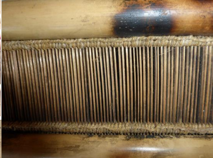
Top left Hand tying the lewi (heddles) for each warp.
