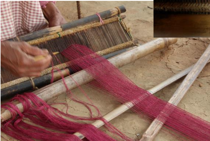
Top left Hand tying the lewi (heddles) for each warp.
