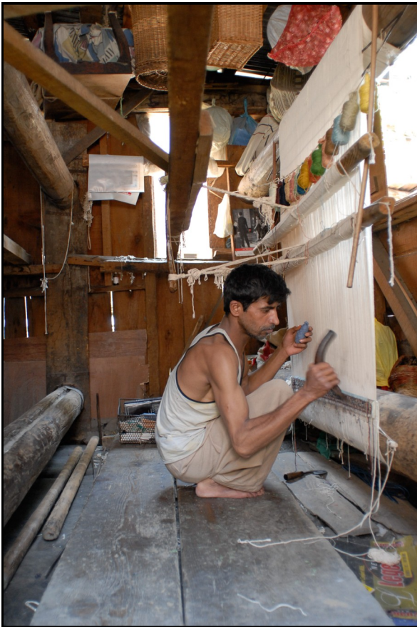
Using a vertical loom, the weaver squats to begin knotting at the bottom end of the carpet. IN his right hand is a toothed instrument to pack the knots and the weft closer together.
