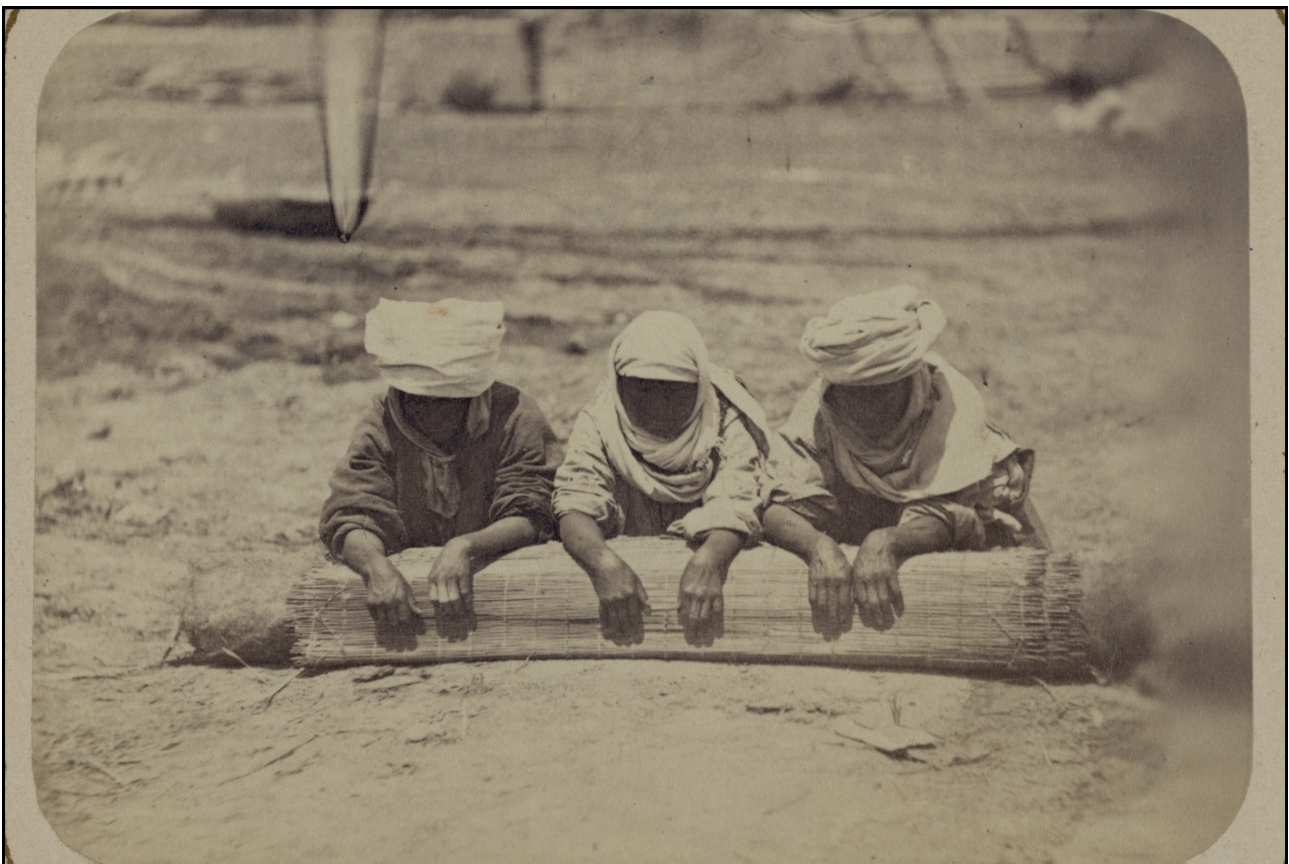
Having rolled the felt into a reed screen, the women turn and pummel it to help the fibres adhere.
